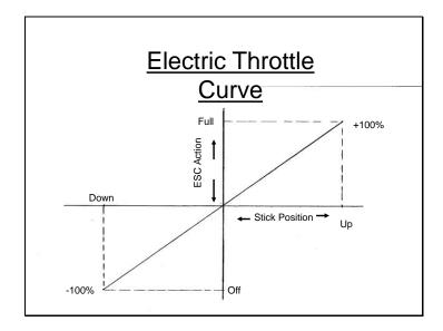
Slide 6 shows a typical throttle curve for an electric model. ESC action is substituted for servo rotation, but the operation is otherwise identical. Shown here is +- 100% throttle range. My experience has shown that this programming procedure will work even though the range is not +- 100%. But, check it out before depending on it.
