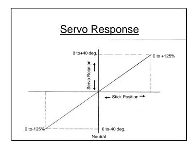
Slide 2 shows the servo response (typically up to 40 degrees or so) as a function of stick position. I will use servo response as the system output for this discussion even though (for electrics) there is no servo on the throttle channel. That way one can visualize what is happening in the throttle channel. The range of 0 to 40 degrees is shown because the transmitter can be adjusted to provide less servo response at the extremes than 40 degrees.
