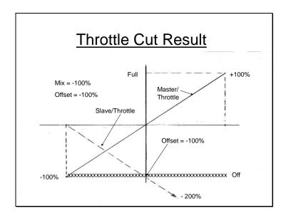
The offset function is used to modify the throttle channel response when the throttle cut function is activated (throttle to throttle mix is on).
